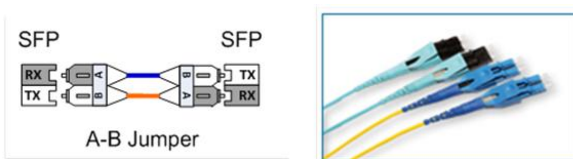
Figure 1: Duplex Fiber Optic Transmission
